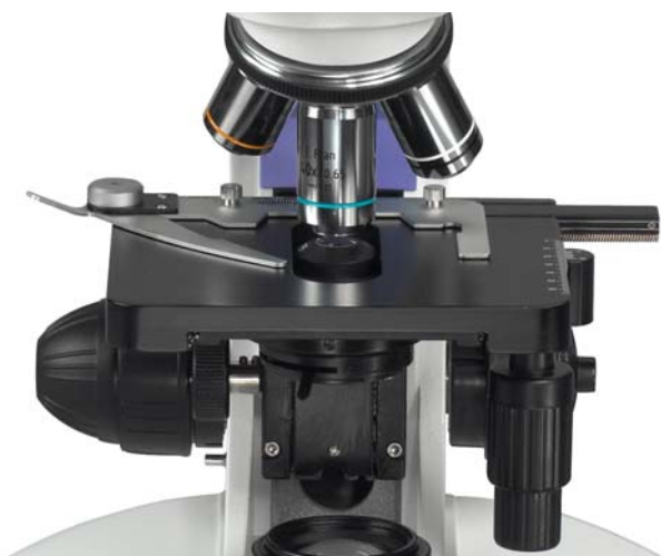
Plan achromat objectives are parfocal and parcentred to minimise refocusing.
