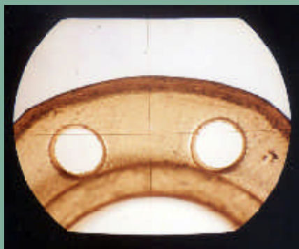
Copper bush viewed at 10x magnification
