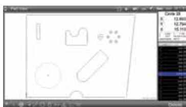
Graphics-based "part view" constructions: Generate popular construction types, like distances and tangent lines, from within the graphical part view itself.
