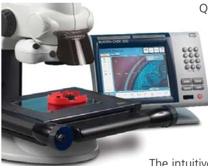
QC-300 features an array of video measurement tools, including simple crosshair measurement, manual or automatic single point detection and multi-point video edge detection.
