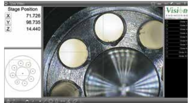
Essential measurement data, with graphics-based "part view" construction displayed alongside high resolution video image. Generate popular construction types from within the graphical part view itself.
