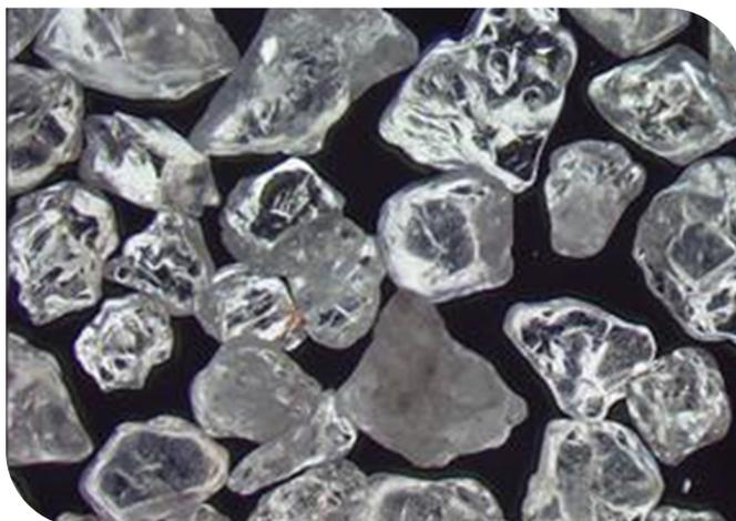
*Sugar crystals under EVO Cam II (100x magnification)*
